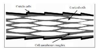
Figure 3. Schematic of a wool fibre showing cuticle and cortical cells.
