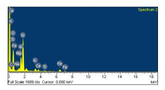
Figure 10. EDX spectra of a sample (mainly soil)
