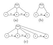
Figure 2: Merging two different models  $(A \rightarrow B \rightarrow C$ and  $D \rightarrow E$ ): a + b = c
