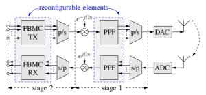
Fig. 2. Proposed reconfigurable TVWS filter bank transmitter (above) and receiver (below) with a polyphase filter (PFF) in stage 1 and a FBMC modulator in stage 2.
