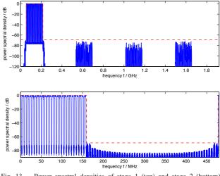
Fig. 13. Power spectral densities of stage 1 (top) and stage 2 (bottom) signals, with spectral masks indicated as dotted lines (US-1).
