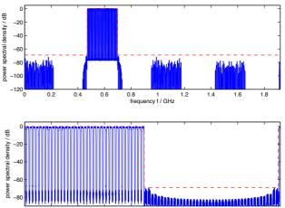
0 50 100 150 200 250 300 350 400 450 frequency f / MHz Fig. 14. Power spectral densities of stage 1 (top) and stage 2 (bottom) signals, with spectral masks indicated as dotted lines (US-2).
