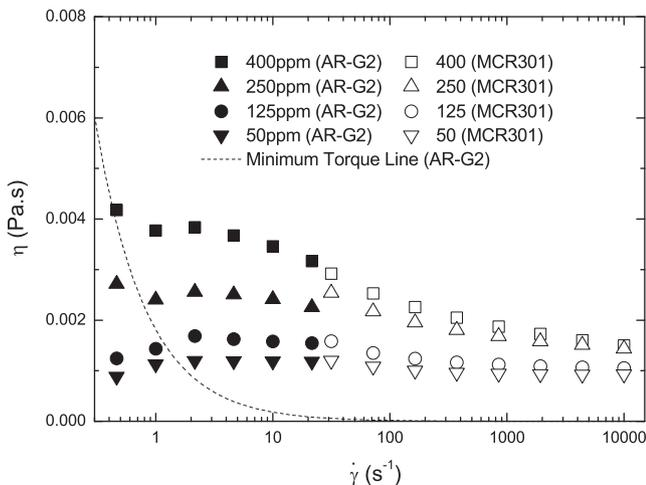
**Fig. 3.** Steady viscosity curves at 20.0 °C for 50 ppm, 125 ppm, 250 ppm and 400 ppm PAA aqueous solutions with 1% of NaCl obtained by a composition of the measurements from cone plate and parallel plate geometries.
