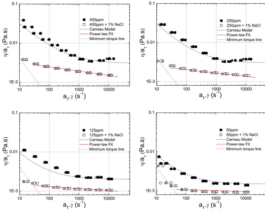
**Fig. 2.** Master viscosity curves for 400 ppm, 250 ppm, 125 ppm and 50 ppm PAA aqueous solutions with and without the addition of 1% of NaCl, carried out at 283.2 (■), 288.2 (▲), 293.2 (●) and 298.2 K (☆). Different symbols correspond to different temperatures, however filled symbols represent samples without salt, and empty symbols represent samples with NaCl.
