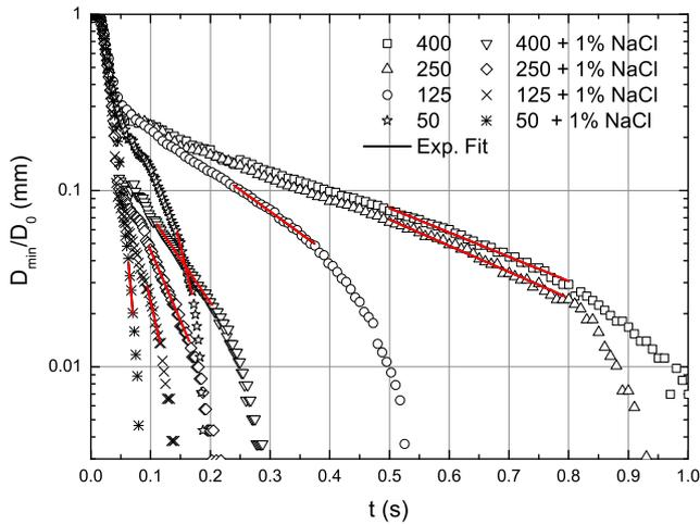
**Fig. 4.** Time evolution of filament diameter in CaBER experiments for 400 ppm, 250 ppm, 125 ppm and 50 ppm PAA aqueous solutions, at 20.0 °C (to improve visually the figure, only part of the experimental data are plotted)
