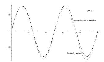
Figure 5. Comparison of iterated and calculated values of y displacement for SO(4)
