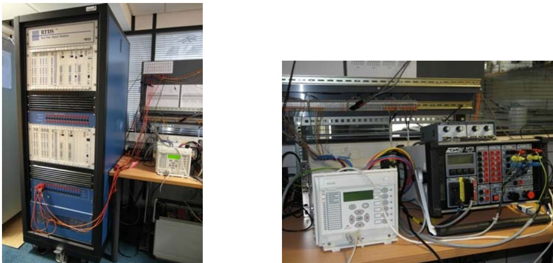
Figure 5-1 Test set-up with real-time digital simulator (left), and protection relay with amplifier (right)
