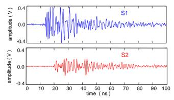
Figure 7: Time-Domain UHF Signals Recorded Simultaneously at Two Sensors
