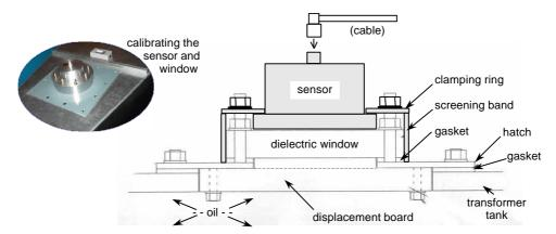
Figure 4: UHF Sensor Assembly on a Transformer Hatch Cover
