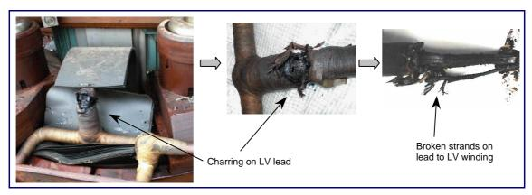
Figure 16: Damaged Joint on 33 kV Lead
