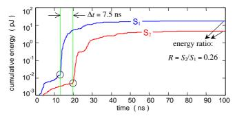
Figure 8: Cumulative Energy Plots Illustrating Parameter Extraction for a UHF Signal Pair
