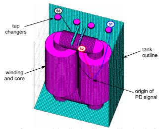
Figure 5: Single Phase Transformer Model Indicating Shortest Signal Paths from PD Source to Sensors
