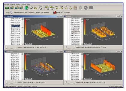
Figure 15: Examples of PD Patterns Recorded at Different Stages During the Monitoring Period
