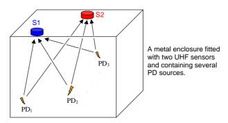
Figure 6: Recognizing Multiple Signal Sources Using Two or More UHF Sensors
