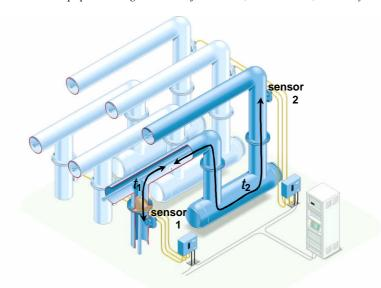
Figure 2: Locating a PD Source in a GIS by the Time-of-Flight Method (*Image courtesy of Diagnostic Monitoring Systems Ltd.*)
