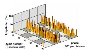
Figure 12: UHF PD Signals from Sensor S1, Phase-Resolved to the 50 Hz Power Frequency
