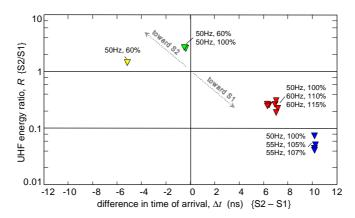
Figure 9: Map of Time-Domain UHF Signal Parameters Showing Multiple Discharge Sources (Specific test frequency and operating voltages [%] are indicated beside each data cluster)
