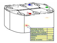
Figure 3: Graphical Interface for Accessing Transformer Monitoring Information
