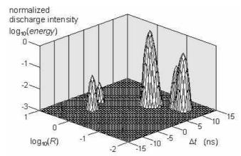
Figure 10: Three-Dimensional Energy-Cluster Map of PD Activity (*Vertical scale shows the signal energy relative to the cluster with the highest energy*)
