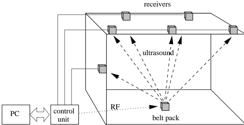
**Fig. 1.** System design setup for automatic followspot tracking [7].
