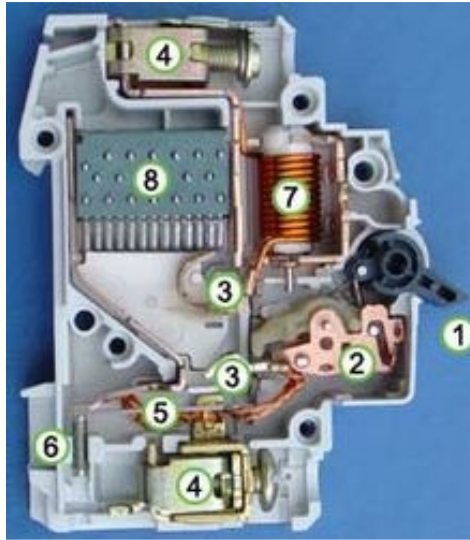
Figure 3: Insides of a mechanically operated circuit breaker [4]
