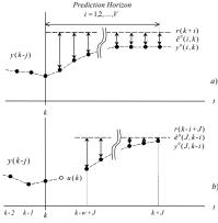
Fig. 1: MPC and Predictive Control Feedback set-ups
