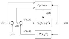
Fig. 2: Structure of the predictive feedback controller
