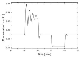
Fig. 5: Open loop responses of the CSTR concentration.
