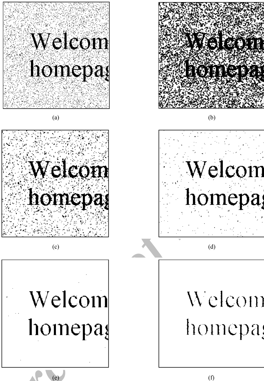
Fig. 2. The example shows a text image corrupted with 10% additive impulsive noise, then filtered with every 5 point rank order filter. It can be seen that rank r = 4 gives a lower MAE than the median. (a) Noisy image, (b) r = 1 dilated image, MAE= 0.392, (c) r = 2 MAE= 0.087, (d) r = 3 median filtered, MAE= 0.012, (e) r = 4 , MAE= 0.008 * optimum, (f) r = 5 eroded image, MAE= 0.029.
