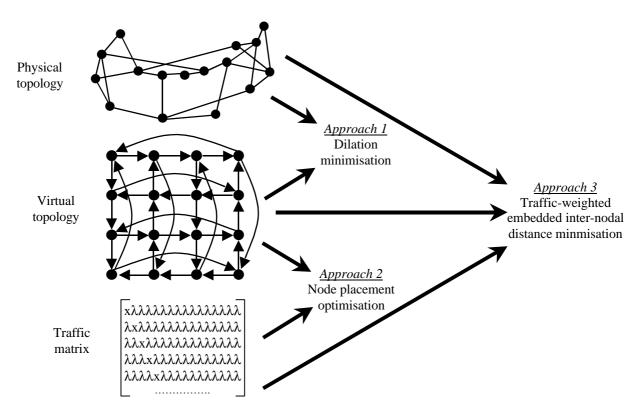
Figure 1 – Three alternative regular virtual topology design approaches
