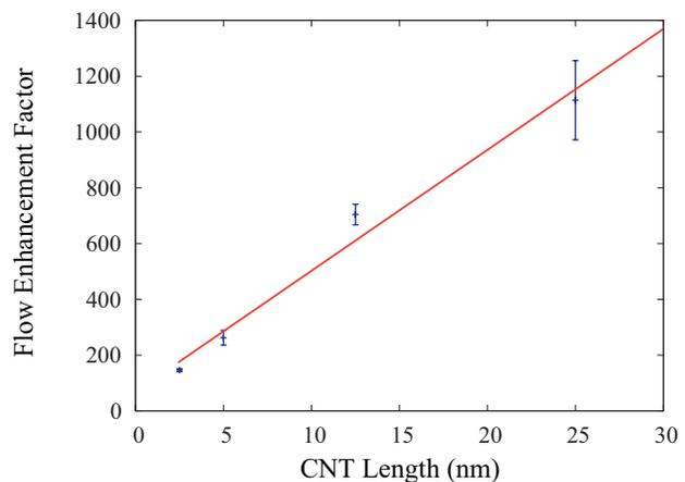
**Figure 4:** Flow enhancement values for different CNT lengths.
