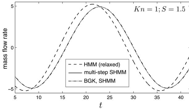
Figure 8: Time evolution of mass flow rate (normalized with the Navier-Stokes prediction of mass-flow-rate amplitude) for  $Kn = 1$  and a timescale separation number,  $S=1.5$ ; fully relaxed HMM solution (dashed line); multi-step SHMM (solid line); full BGK solution and SHMM (dashed and dotted line)
