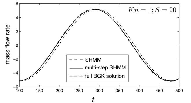
Figure 7: Time evolution of mass flow rate (normalized with the Navier-Stokes prediction of mass-flow-rate amplitude) for  $Kn = 1$  and a timescale separation number,  $S=20$ ; SHMM (dashed line); multi-step SHMM (solid line); full BGK solution (dashed and dotted line).
