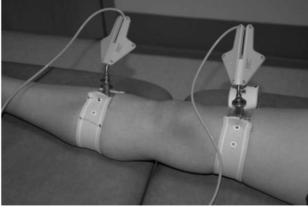
External tracker mountings with adjustable straps 100x66mm (150 x 150 DPI)
