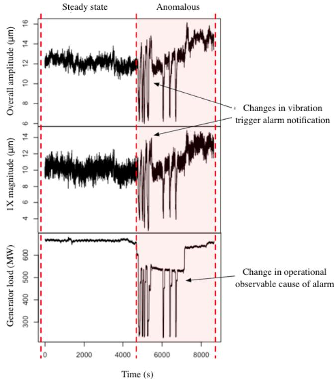
**Figure 1. Example routine alarm, in which a transient in generator load has induced a vibration change. This correlation has to be manually identified from a variety of operational observables after the prompting of an alarm.**
