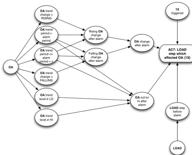
**Figure 3. Inference diagram showing the forward chaining nature of the symbolic rules, corresponding to features within the continuous data. This particular example is for a load step change, causing a change in the overall amplitude.**
