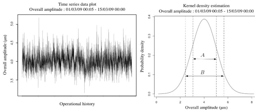
**Figure 5. Steady-state overall amplitude data (left), with corresponding kernel estimation (right). From the resulting unimodal distribution, the envelopes of normal operation and trend tolerances can be defined for the limit profile.**
