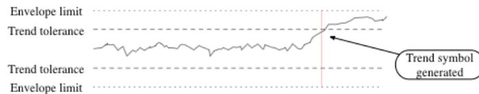
**Figure 4. Example time series data illustrating calibrated tolerance and limit settings. The breach of the trend tolerance boundary with continued transient behaviour represents the criteria for generating a trend symbol to the KBS. The envelope limit corresponds to an excessively high/low level within the inference base.**
