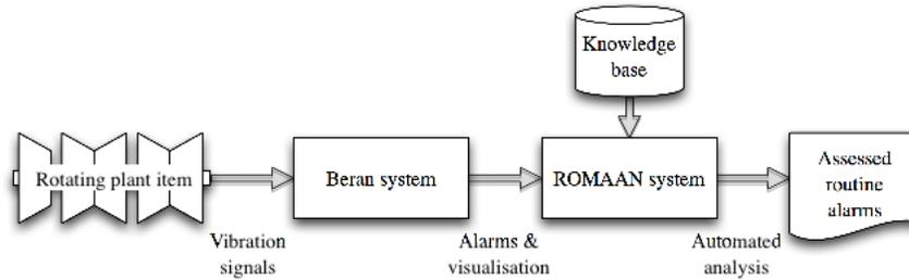
**Figure 2. Schematic of the knowledge-based prototype system in use, which provides automatic decision support for turbine generator alarms**
