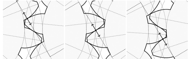
Fig. 25 Moving of contact point along the pressure line (shown by movement of arrow)
