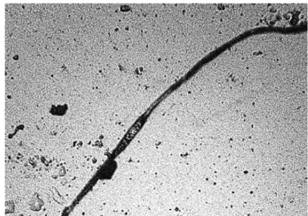
Fig. 22 Cutting wear particle [56]
