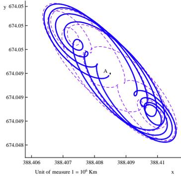
Figure 9: The bounded orbit around A; the blue, continuous line is the numerical integration of the nonlinear system, the purple, dashed line is the analytic solution of the linearized system.
