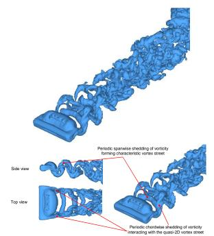
Figure 5: Wake geometry expressed as vorticity isosurface for the rectangular wing positioned normal to the flow
