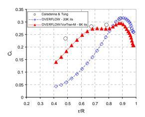
Figure 15: Comparison of measured and predicted spanwise loading ( $C_{T \ Experiment} = 0.0046$ ,  $C_{T \ OVERFLOW} = 0.00432$ ,  $C_{T \ OVERFLOW/VorTran=M} = 0.00458$ ) from [50]
