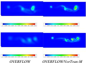
OVERFLOW OVERFLOW/VorTran-M Figure 12: Predicted vorticity magnitude for a 1-bladed rotor in forward flight on a plane perpendicular to the direction of flight, 33 (upper) chord lengths and 40 (lower) downstream of the hub.  $\Delta s_{OVERFLOW} \approx 0.43c$  and  $\Delta s_{VorTran-M} \approx 0.87c$
