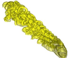
Figure 9: CGE/VorTran-M prediction of a LPD-4 class ship airwake
