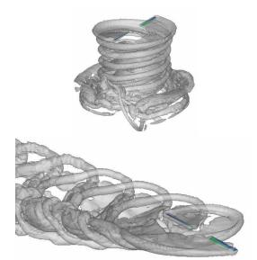
Figure 7: RSA3D/VorTran-M rotor wake predictions: two bladed untrimmed rotor in slow speed ascent (upper) and two bladed untrimmed rotor in forward flight (lower)
