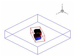
Figure 13: 2-bladed rotor and hub grid arrangement. Blade grids (black), tip-caps (blue), root-cap (red), hub grid (green), bounds of initial VorTran-M grid (blue line) and grid on which VorTran-M sets boundary conditions (red line)
