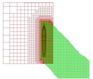
Figure 8: Intersection of Cartesian grid (red) and VorTran-M grid (green) at right for a yawed flow condition
