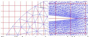
Figure 18: Intersection of unstructured (blue) and VorTran-M grids (red) at left and center
