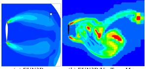
(a) FUN3D (b) FUN3D/VorTran-M Figure 17: Mid-plane vorticity magnitude predicted by the FUN3D/VorTran-M coupled simulation for the NACA0012 wing at 90° angle of attack
