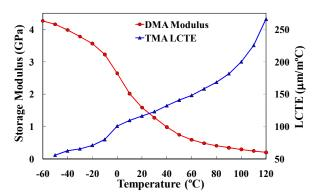
Figure 8 PP matrix properties versus temperature.
