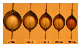
Figure 1 Micrographs of a GF-PP microbond sample heated at 220°C in air.
