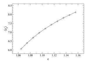
Fig. 3 Mean number of neighbours  $\langle z_{\rm s} \rangle$  within a range defined by the cutoff value c for the potentially stable particles. The data are based on five imaged volumes with a volume fraction  $\phi=0.608\pm0.004$ . The line, in this and subsequent figures, is a guide to the eye.
