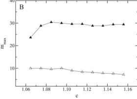
Fig. 9 (A) Mean bridge size  $\langle m \rangle$  as a function of cutoff c for all bridges (black circles) and for only bridges of size m > 1 (red diamonds). Results are shown for the LCOM (open symbols) and LSQS (filled symbols) criterion. (B) Maximum bridge size mmax for LCOM (open triangles) and LSQS (filled triangles). Sample as in Fig. 3.
