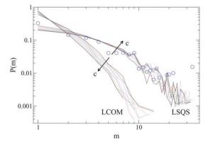
Fig. 8 Bridge size distribution P(m) for different cutoff values c in the range  $1.05 \le c \le 1.14$ , for the LCOM and LSQS stabilising subset selection criteria (as indicated). The colours and line styles are for clarity only; the evolution with increasing cutoff c is monotonic in c in both cases. Sample as in Fig. 3. The circles indicate P(m) for a simulated granular sample (see text).
