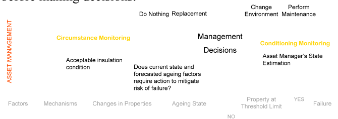
Fig. 1. Crucial information for an assets manager acquired from circumstance and conditioning monitoring
