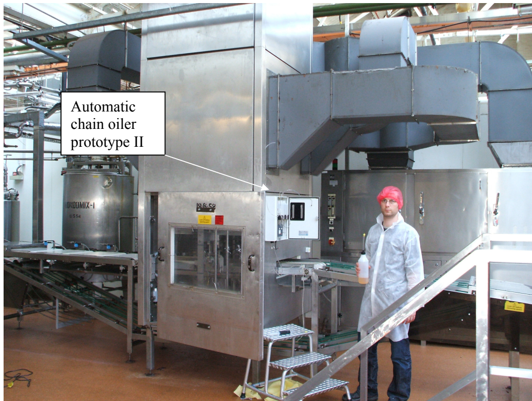
Figure 6-11 Installation of the second oiler prototype on the same machine as the first. This time mounted on the outside for easier access.
