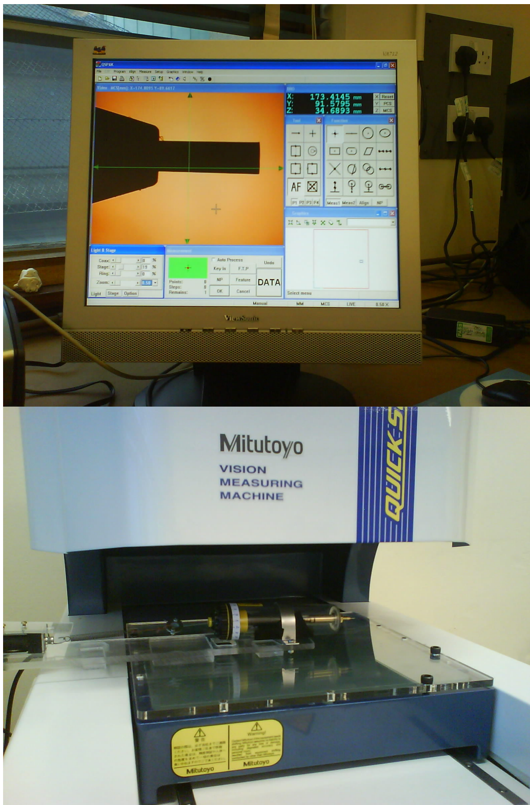
Figure 4-18 Measuring valve needle displacement using a Vision Measuring Machine, VMM. The top image shows the gauge rod inserted into the valve so that contact is made with the needle.
