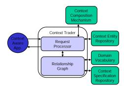
Fig. 2. The structure of a context trader.
