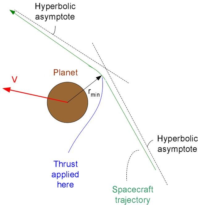
Fig. 2. Illustration of a gravity assist manoeuvre
