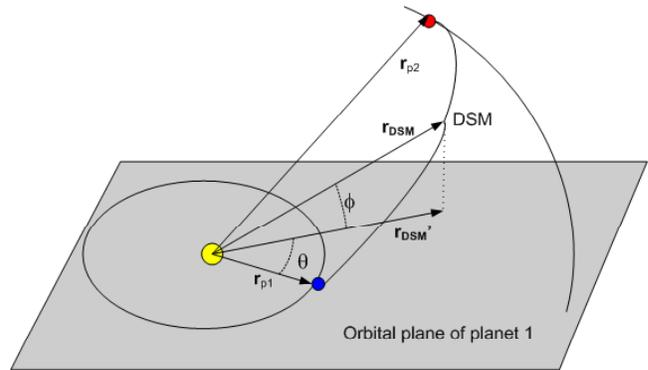
Fig. 1. Mission leg model with a deep space manoeuvre
