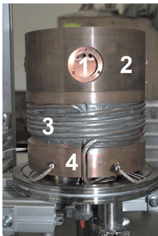
FIG. 3. (Color online) The copper construction affixed atop the bottom flange of the vacuum chamber and isolated from the external environment by insulating “feet” constructed from PEEK. Label 1 shows a glimpse of the reservoir via the entrance portal for the firing system (see Sec. II C); label 2 identifies the radiation shield; label 3 indicates the copper tubing for the LN 2 ; and label 4 highlights the thermal block.
