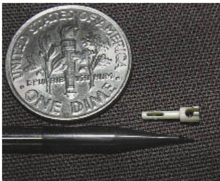
*JLP Machine employed a 0.015"-dia. Microcut ball mill to machine features, including a 0.015"-wide slot, on a tiny medical component made of polyetheretherketone (PEEK) polymer. Photo courtesy JLP Machine.*
