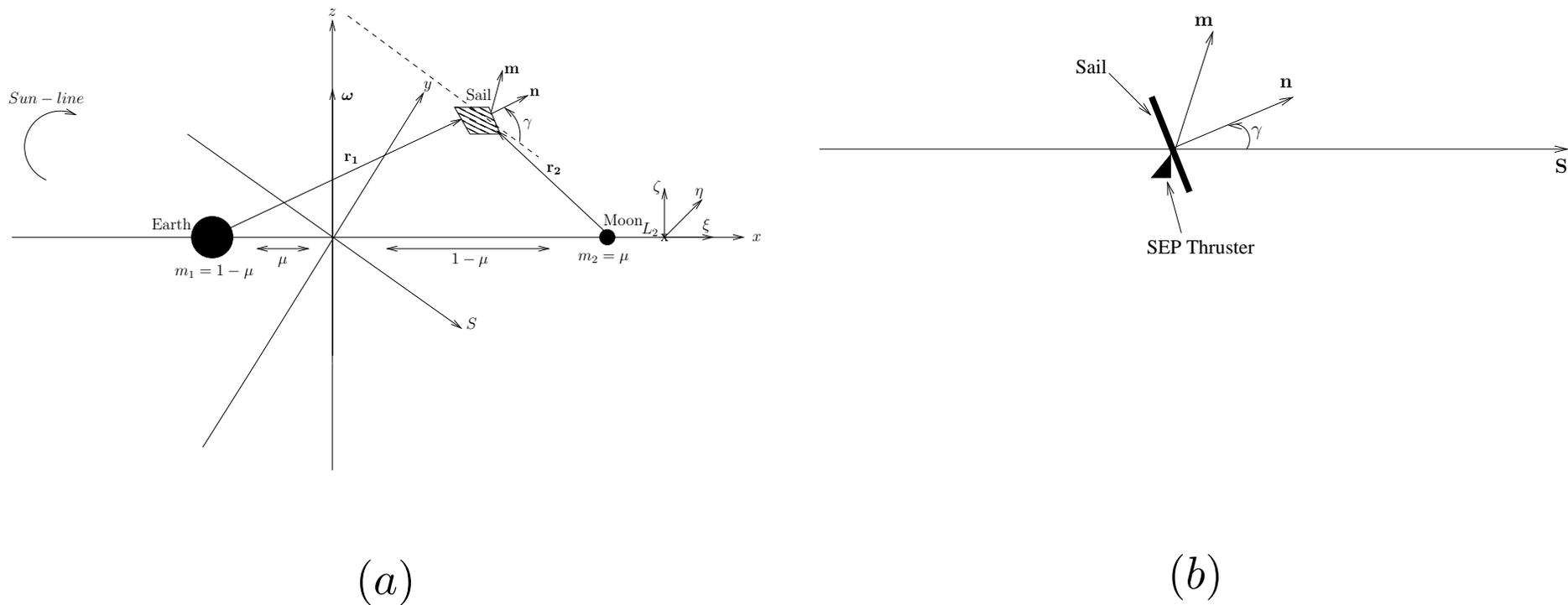
Figure 1: (a) Schematic geometry of the Hybrid Sail in the Earth-Moon restricted three-body problem; (b) Angle  $\gamma$  between the Hybrid Sail surface  $\mathbf{n}$  and the Sun-line direction  $\mathbf{S}$ , and SEP thrust vector direction  $\mathbf{m}$ .
