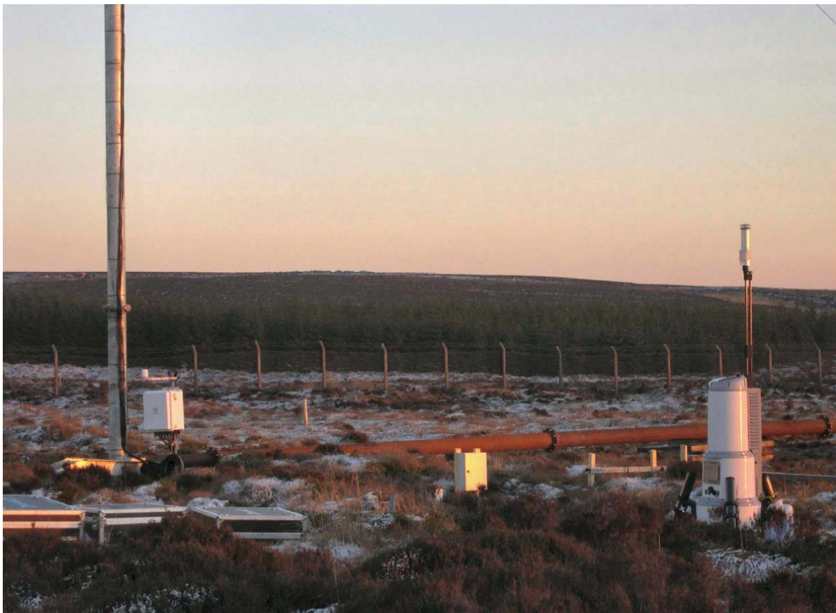
Figure 3. NPC/QinetiQ ZephIR Lidar co-located with mast.
