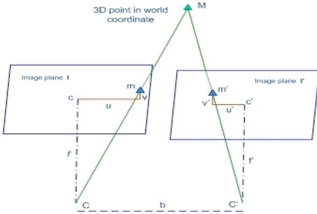
Figure 3 - Disparity estimation using Stereo-pair images
