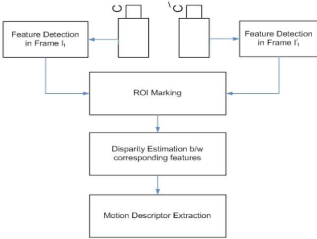
Figure 1 – Block diagram of motion descriptor extraction using stereo-pair footage
