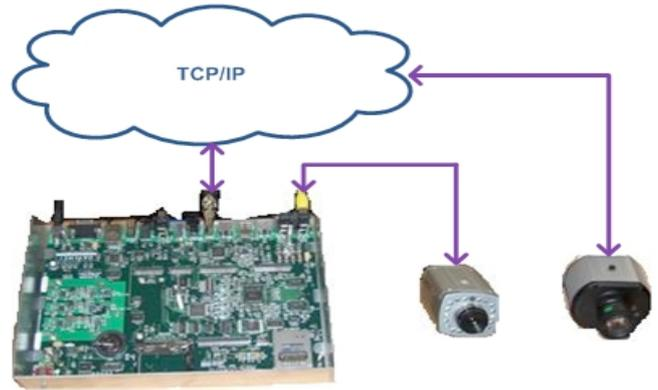
Figure 8 – Proposed DM6446 layout with IP & analogue Cameras
