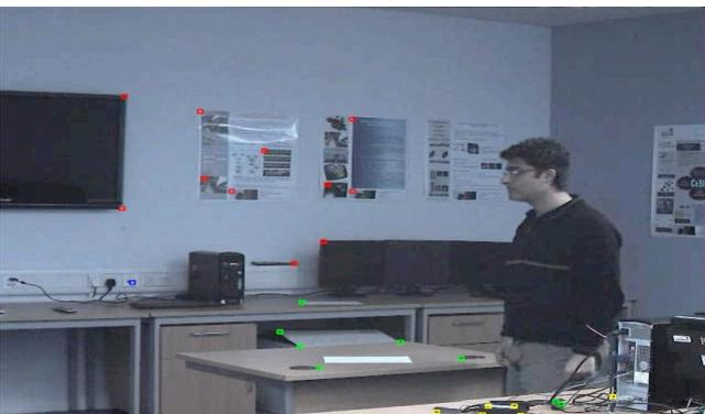
Figure 7 - Frame from camera 1, showing depth of selected feature points. Red showing farthest then blue, green and yellow nearest
