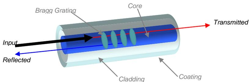
Figure 4: Illustration of a Fibre Bragg Grating
