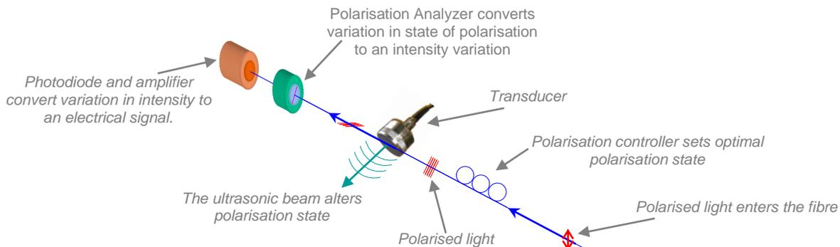
Figure 1: Polarimetric Detection System
