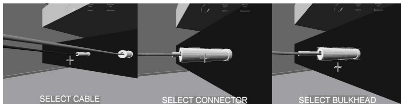
Figure 9. VR user interface for assembly planning
