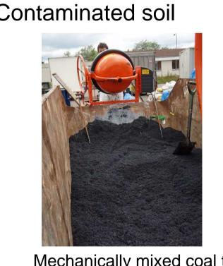
Mechanically mixed coal tar in sand or field-obtained contaminated soil
