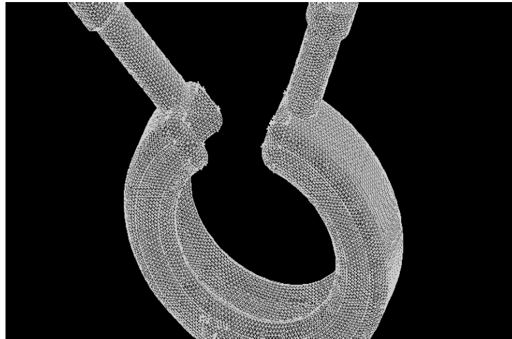
FIGURE 10. Casing Fluid Region Tet Mesh
