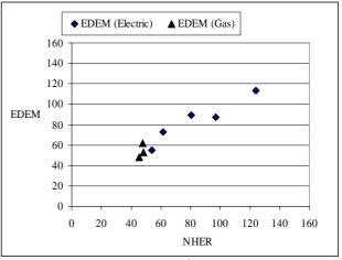
Figure 1:  $CO_2$  emissions (kg /m<sup>2</sup> yr) – EDEM vs. NHER Surveyor.
