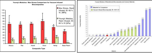
Fig. 4: Young's Modulus/ Maximum stress for vacuum infused biocomposites
