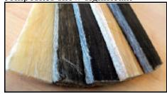
Fig. 3: From left to right, Sisal, Flax, Hemp, Abaca and Kenaf composites
