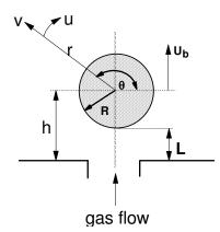
If the bubble volume is taken as a control volume, as shown on Fig. 1, the application of the conservation of mass leads to the following equation, assuming constant density conditions
