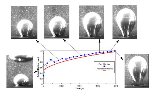
Figure 5 Comparison of experimental and predicted bubble radius
