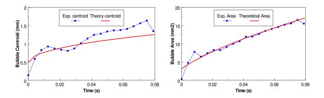
Fig. 6 Theoretical and exp. centroid position Fig. 7 Theoretical and exp. bubble area
