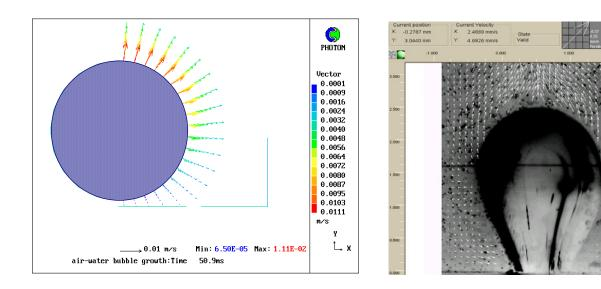
Fig 8b Experimental and predicted vector field at 50 msecs<sup>1</sup>
