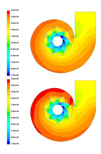
Figure 6: Numerical pressure contours in two different time steps
