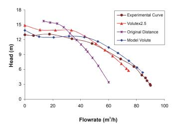
Figure 3: Characteristic curve
