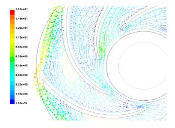
Figure 7: Relative velocities inside the impeller
