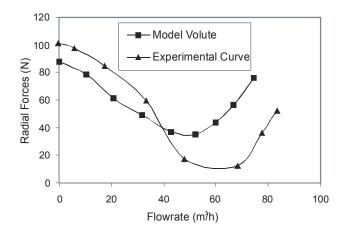
Figure 5: Experimental and numerical radial forces
