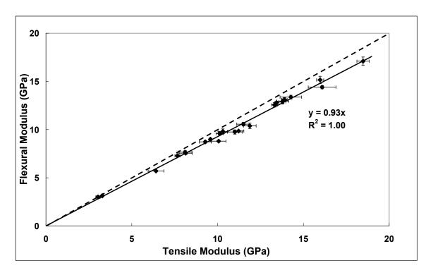
Figure 5 Flexural versus Tensile Youngs' modulus
