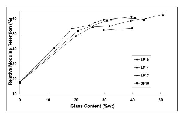
Figure 7 Modulus retention after 24 hour boiling versus fibre content
