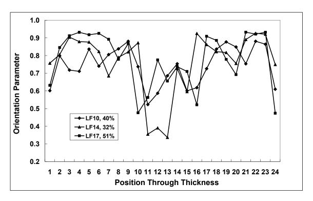
Figure 11 Fibre orientation parameter across sample thickness
