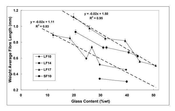
Figure 3 Residual weight average fibre length versus fibre content
