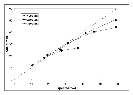
Figure 2 Comparison of measured and calculated glass contents
