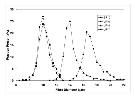
Figure 1 Fibre diameter distributions of input fibre products
