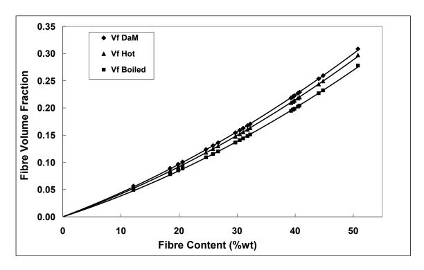
Figure 10 Fibre volume fraction versus weight fraction
