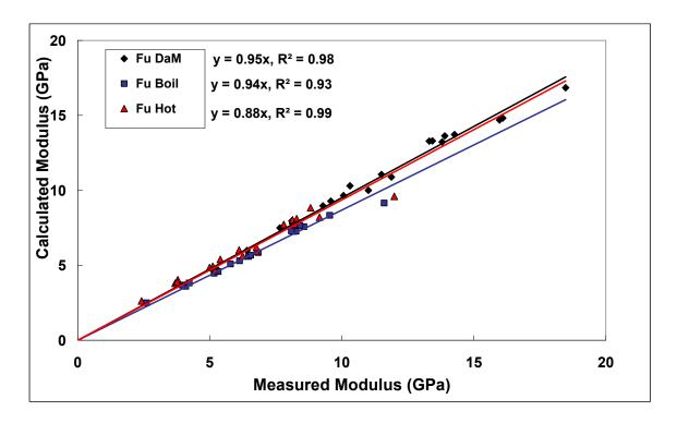
Figure 14 Comparison of Fu-Lauke model predictions against experimental values
