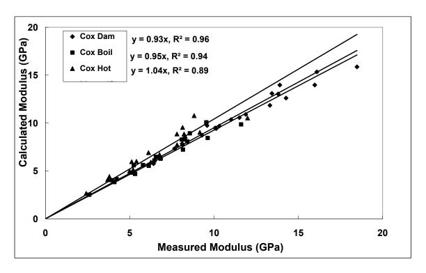
Figure 13 Comparison of Cox-Krenchel model predictions against experimental values
