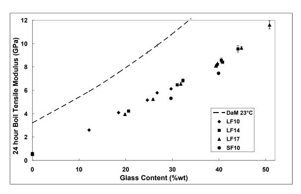
Figure 6 Young's modulus after 24 hour boiling water conditioning
