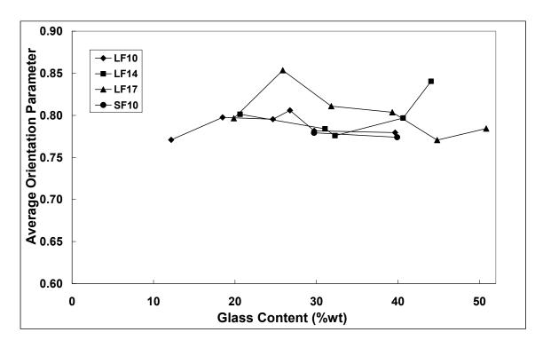
Figure 9 Fibre orientation parameter from optical analysis
