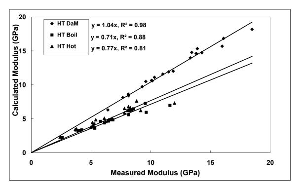
Figure 12 Comparison of Halpin-Tsai model predictions against experimental values
