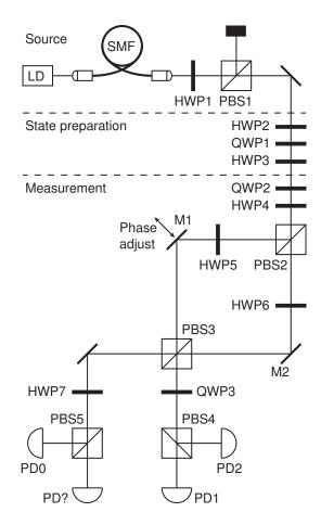
FIG. 1: Experimental apparatus. LD=Laser diode, SMF=single mode fiber, PBS1-5=polarizing beamsplitters, HWP1-7=zero-order half waveplates, QWP1-3=zero-order quarter waveplates, PD0-2, PD?=amplified photodiodes
