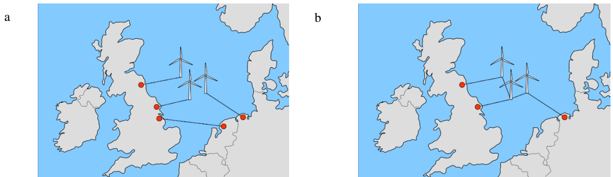
Fig. 1 Potential North Sea offshore wind connection, (a) point-point, (b) multi-terminal.
