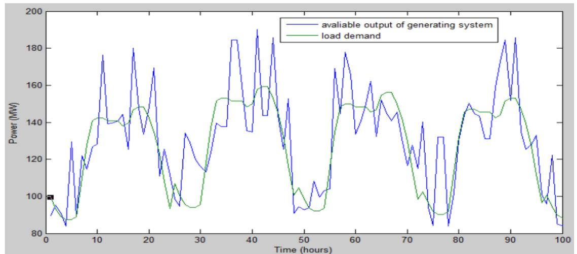
Figure 4. Curve of load demand and available generating power capacity.
