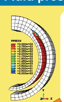
The moisture swelling process is not uniform and develops from the surfaces which are subject to fluid. Adsorption, which governs the progress of swelling can occur only at open surfaces. Therefore, the fluid pressure penetration technique needs to be involved into simulation. This is an automated application of fluid pressure dependent on changes of contact conditions.
