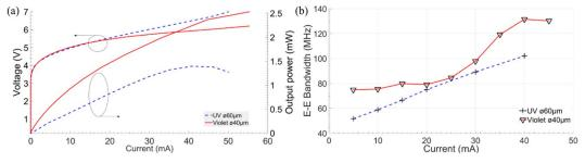
Figure 1 - (a) output power and voltage vs. current and (b) electrical -3dB bandwidth versus current for UV and violet µLEDs
