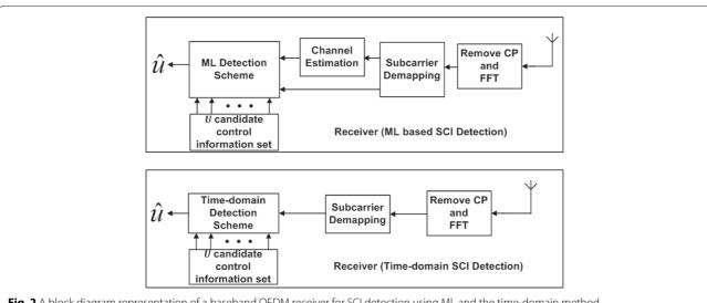
Fig. 2 A block diagram representation of a baseband OFDM receiver for SCI detection using ML and the time-domain method
