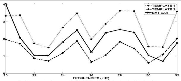
Fig. 4. Maximum value of beam pattern's main lobe associated with Templates 1 and 2 and R. leschenaultii's ear.
