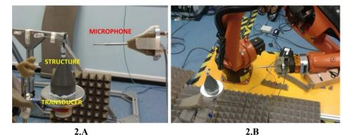
Fig. 2 Beam pattern measurement: (A) Microphone recording sound from the transducer and through the receiver structure; (B) KUKA robot controlling microphone position around the receiver structure.
