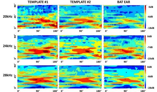
Fig. 3. Contour plots depicting the receivers' beam patterns over azimuth and elevation angles (degrees) and for frequency values 20kHz, 24kHz and 28kHz. The azimuth and elevation intervals correspond to the quarter of sphere in front of the upper opening of each receiver.
