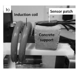
The patch sensor was left uncovered in air or covered with surface water, dry sand, wet sand or wet soil. The instrumented concrete block was then heated by a two-turn induction coil, as shown in Figure 1b. The current within the coil was driven at 100 - 200 A amplitude and 350 kHz frequency for 15-20 seconds.
