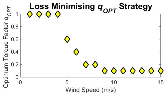
Fig. 5.  $q_{OPT}$  Strategy to Minimise Generator Losses
