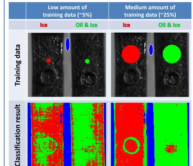
$\succ$  HSI empowered by signal processing is able to distinguish pure ice from oil under thin ice layer
