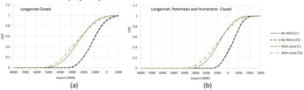
Figure 6: cumulative distribution for 'Longannet Closed' and 'Low Conventional' cases estimated by convolved and time series analysis (denoted C and TS respectively) with and without the existing wind fleet.
