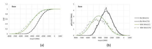
Figure 5: (a) cumulative and (b) density plots of convolved and time series estimations (denoted C and TS respectively) of boundary import requirements for the base case scenario with and without wind.
